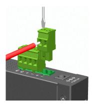
If cascading the power to next device is needed, install the power wires and plug for another switch. Then, use DC2 contacts.
